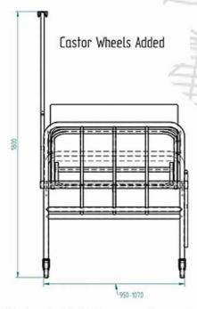
Bed Legs: 32 x 2mm Round Tubing Cold Rolled
